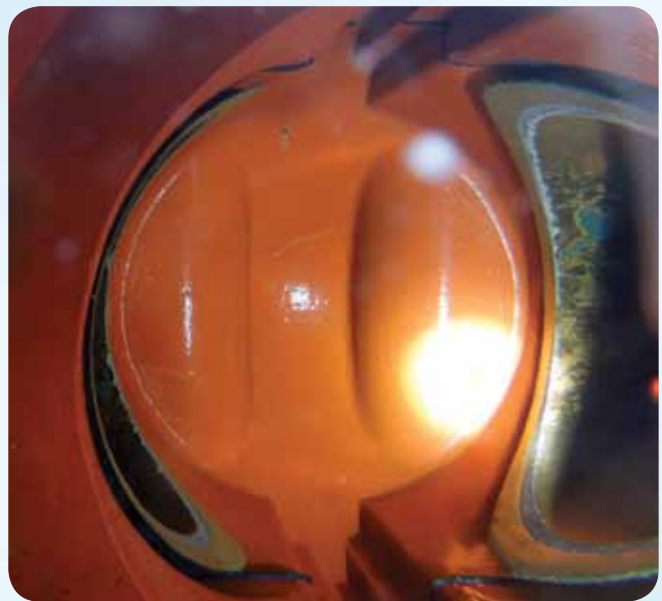
An under-pressure look of clean valve seat.
