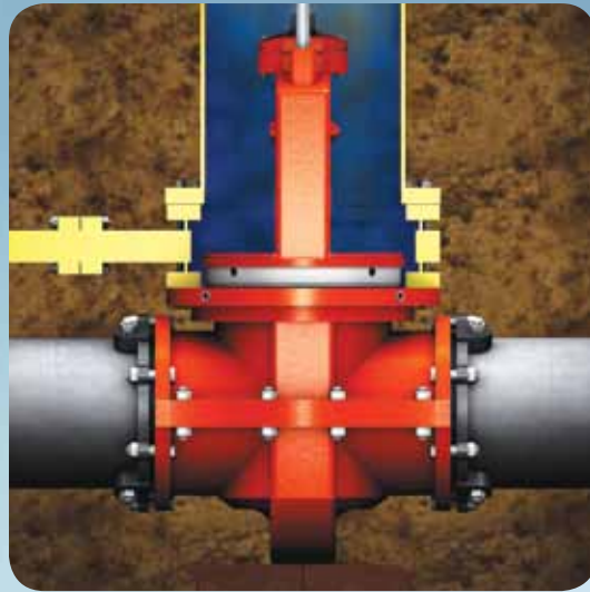
Step 2 Insert bonnet into the valve body.
